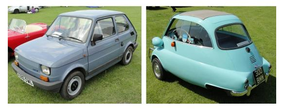
As a microcar is generally classed as having no more than three cylinders and a displacement of not more than 700cc there are a number of Italians which fit the bill, the Fiat 500 and its successor the 126 being the most obvious and recent, although the Isetta bubble car is perhaps the model which is more likely to spring to mind in this context.
